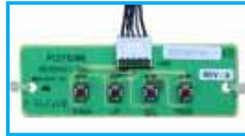
Push Button Control Board
